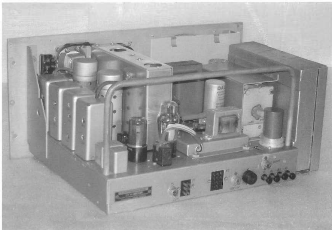
Rear view of the RV9A. The power supply unit is fitted in the centre of the chassis
