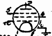
ARP12 base connections
