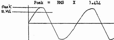
As we get on the higher frequencies, condensers and coils (chokes) get up to funny tricks. While not dissipating heat, they tend to reduce the current in a circuit: this is called their <u>reactance</u>.
